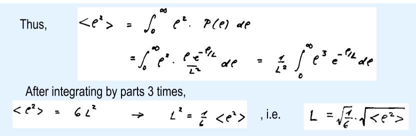
*Diffusion length*  $\propto$  square root of the avg. squared distance at which a neutron is absorbed ... There are many scattering events (~  $\lambda_t$ ) that have occurred before
